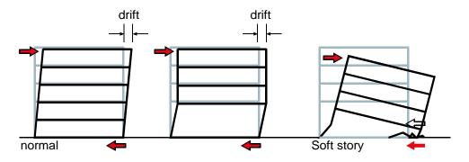
Fig 2.5 (a) Soft Storey due to Excessive Floor Height in Ground Storey
