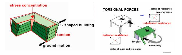
Fig 2.8 Effect of Torsion in Building
