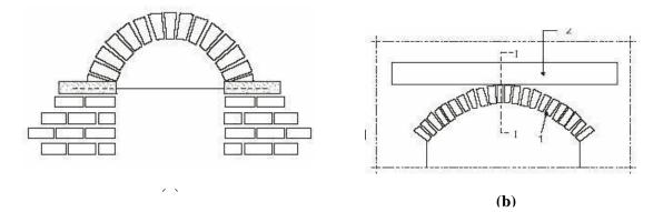
Fig 4. Strengthening of Arches (IAEE, 1984)
