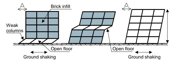
Fig 2.5 (b) Soft Storey due to Open Floors
