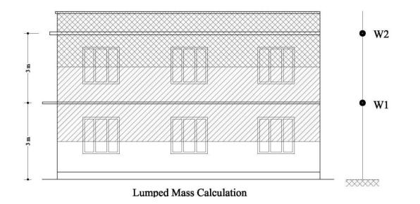
2.6 Calculation of Earthquake Load (*Referring NBC 105*)
