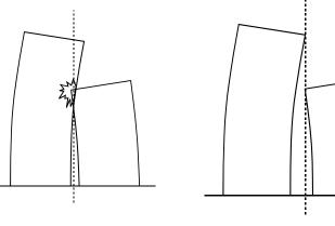
Fig 2.2 (a): Different Floor Height Buildings Suffer More in Pounding Fig 2.2 (b): Pounding due to Small Gap of Two Buildings
